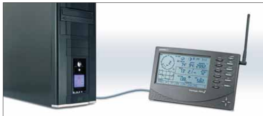
The Davis Vantage Pro2 Plus weather station is comprised of an indoor console and outdoor integrated sensor suite (ISS). There is also an optional upgrade (known as Weatherlink (pictured)) that allows all the readings to be logged and transferred to a PC in standard CSV format.
