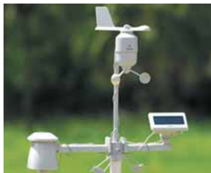
The Oregon Scientific WMR200 wireless weather station can communicate with external sensors located up to 100m away, via 433MHz RF transmission (open space).
